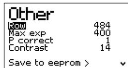
Row is the sensor row used for measuring wavelength. The maximum exposure time (in milliseconds), pressure measurement correction, and screen contrast can also be changed. Note that there is no value range checking; consult the command language in appendix D for more information. Alter values as above.
