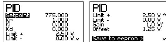
The MWM can output a PID control signal on the SMA connector for laser wavelength stabilisation (see 4.3.4). The PID menu allows display and adjustment of the PID setpoint, gain coefficients, offset voltage and limits. These values would normally be entered using *mogwave* or other interface but it may be useful to display and make small changes on the device.
