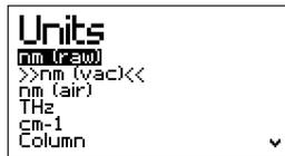
The MWM measures wavelength in ambient conditions, but uses measured temperature and pressure to estimate the wavelength in vacuum, in air at standard temperature and pressure, or as a frequency or wavenumber. *Column* returns the sensor pixel number corresponding to the spectral peak, for diagnostic purposes.
