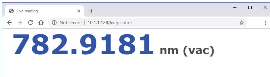
Figure 3.3: Live view, showing the wavelength in real time.
