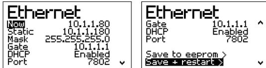
The ethernet sub-menu shows the current IP address, and stored (static default) values for static IP address, netmask, gateway DHCP and TCP/IP port.
