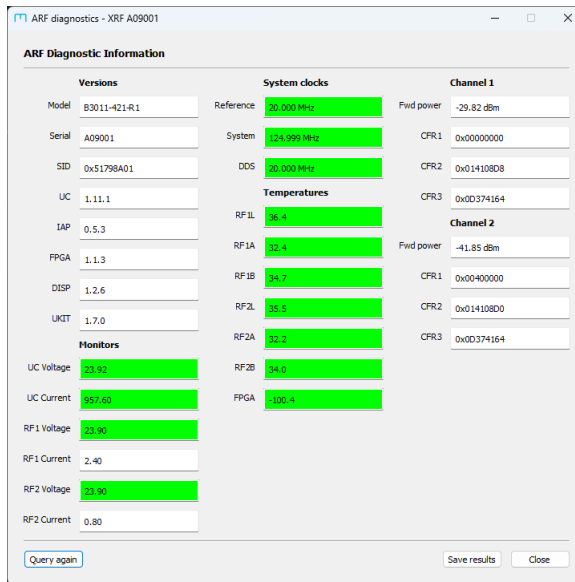
Figure 4.7: Diagnostic information about the connected XRF unit, which should be sent to MOGLabs for analysis if there is a problem with the device.
