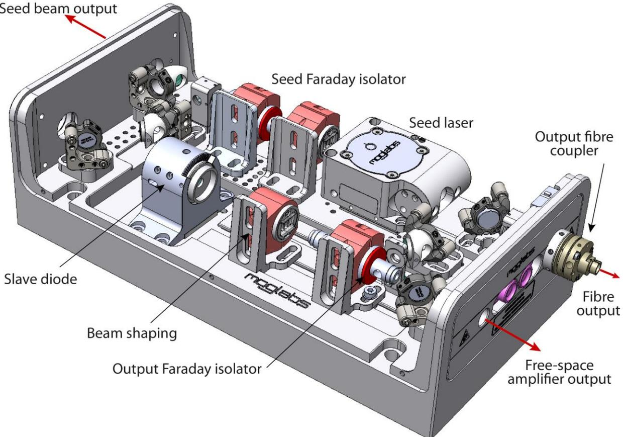
Two outputs are available: the main amplified beam, and a secondary beam of unused output from the seed laser. The plots at right show the main free-space output for 399nm and 461nm: 300mW and 800mW, after isolator. An additional 100 and 200mW are available from the secondary seed beams, which might be used for frequency-locking, or imaging.
