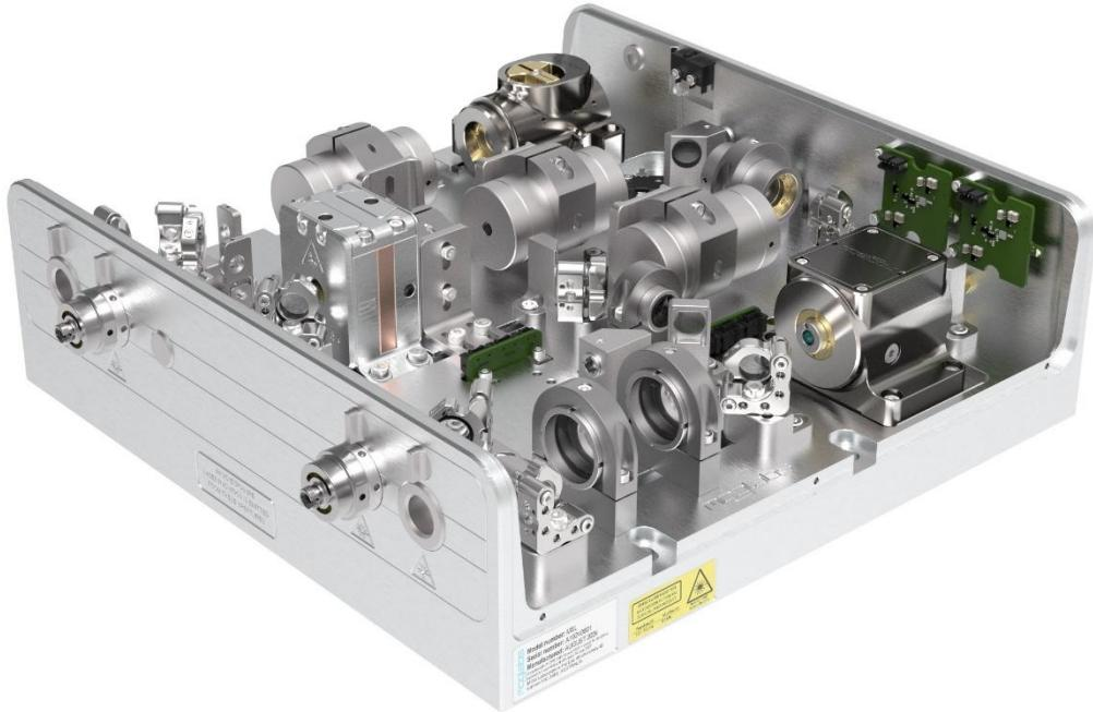
The MOGLabs MSHG seed + amplifier + linear cavity SHG system is a compact, higher power alternative to our standalone linear cavity SHG system with external seed + amplifier offering. The MSHG combines our unique cateye seed laser with a high power tapered amplifier and a linear enhancement cavity to generate ultra narrow linewidth, high power visible light from 370-665nm.
