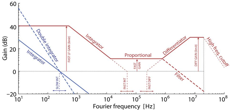
**Figure 1.3:** Conceptual Bode plot showing action of the fast (red) and slow (blue) controllers. The slow controller is either a single or double integrator with adjustable corner frequency. The fast controller is PID with adjustable corner frequencies and gain limits at the low and high frequencies. Optionally the differentiator can be disabled and replaced with a low-pass filter.
