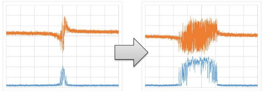
**Figure 3.2:** Scanning the laser with P-only feedback on the fast output while scanning the slow output causes the error signal (orange) to become extended when the sign and gain are correct (right). In a PDH application, the cavity transmission (blue) will also become extended.
