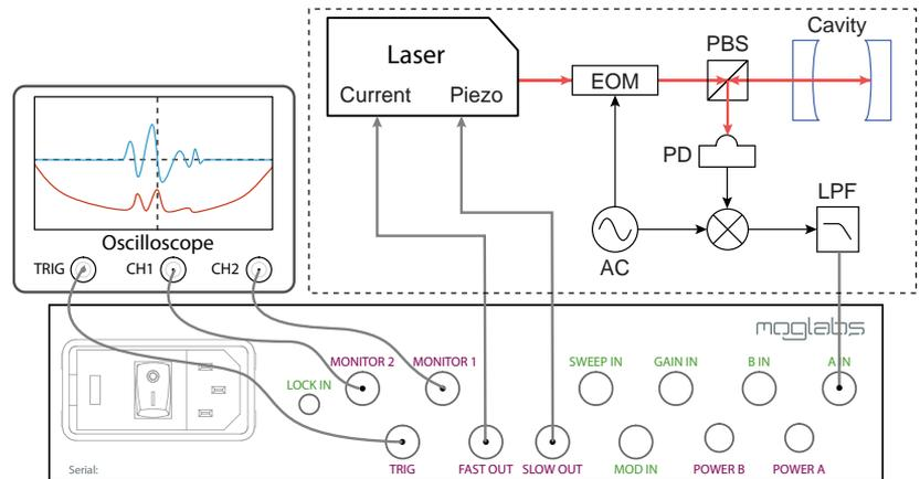
**Figure 3.1:** Simplified schematic for PDH-cavity locking using the FSC. An electro-optic modulator (EOM) generates sidebands, which interact with the cavity, generating reflections that are measured on the photodetector (PD). Demodulating the photodetector signal produces a PDH error signal.
