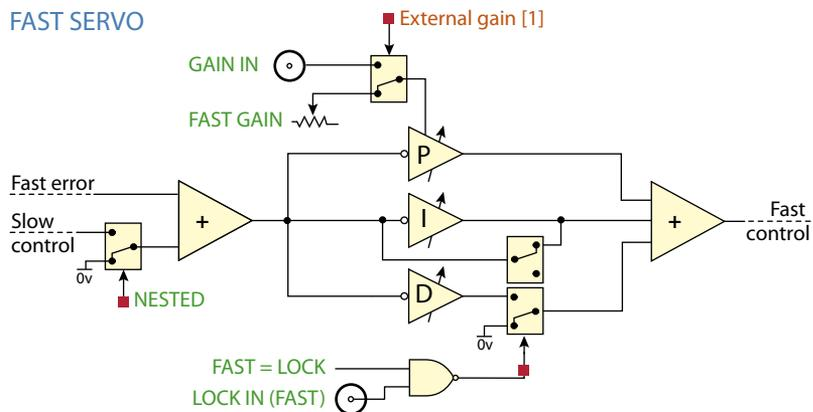
**Figure 1.7:** Schematic of fast feedback servo PID controller.
