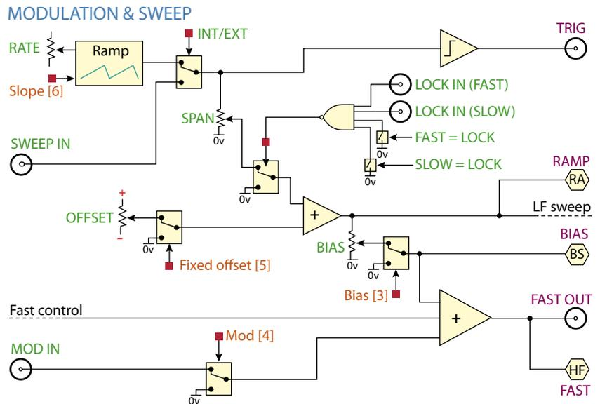
**Figure 1.8:** Sweep, external modulation, and feedforward current bias.
