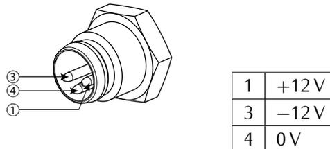
Figure 2.1: M8 connector pinout for POWER A, B.
