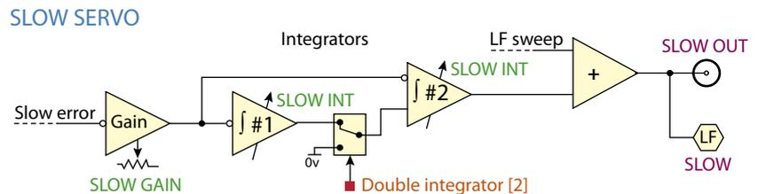
**Figure 1.6:** Schematic of slow feedback  $1/I^2$  servo. Hexagons are monitored signals available via the front-panel selector switches.
