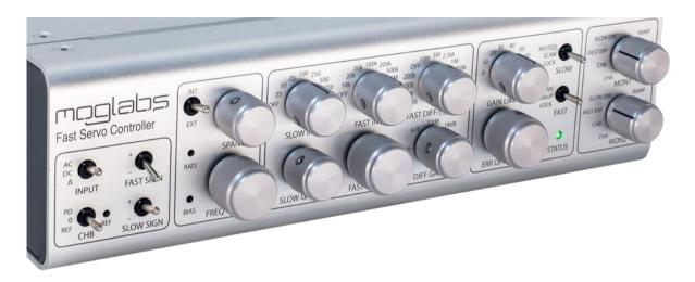
The MOGLabs FSC fast servo controller provides high bandwidth low latency PID/PI<sup>2</sup>D feedback control for linewidth narrowing and frequency locking with a high-finesse optical cavity.
