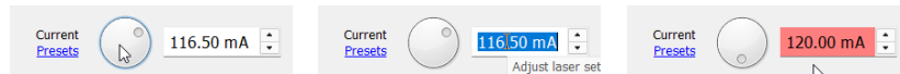
Figure 4.4: Virtual encoders can be smoothly adjusted by mouse-dragging horizontally on the dial (left), scrolling the mouse-wheel, or changed to a new value by typing in the box (middle). When the parameter hits a limit on its permitted range, the background colour changes to red (right).
