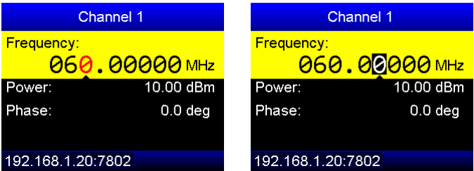
Figure 2.3: The basic parameters of each channel can be edited directly. Turning the encoder wheel modifies the selected digit of the current value (left) as indicated by the arrow. Pressing the encoder wheel changes to digit select mode (right), allowing the selected digit to be changed by turning the encoder.
