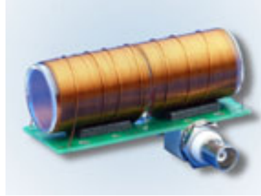
Figure C.1: Vapour cell, Zeeman coil, and primary excitation coil, mounted on PCB (available from MOGlabs).
