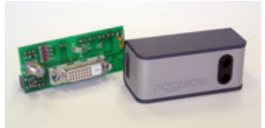
Figure 1.1: The MOGlabs DLC is readily connected to a laser diode, temperature sensor and thermo-electric cooler via the provided laser head board.
