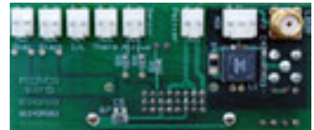
Figure F.1: MOGlabs DLC laser head board showing headers for connection of laser diode, piezo actuators, temperature sensor, TEC and head enclosure interlock.
