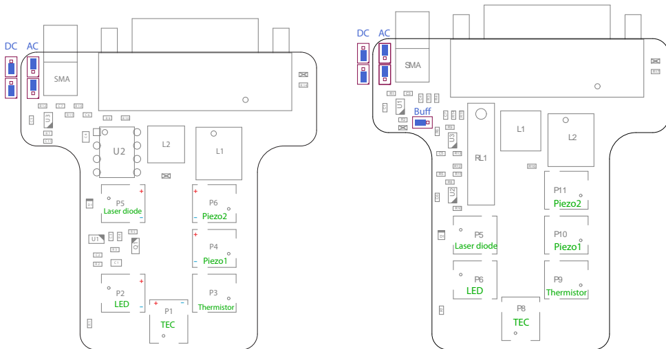
Figure B.3: B1047 (left) and B1240 (right) enhanced laser head boards. Jumpers at top left can be configured for AC or DC coupling. The B1240 has an additional jumper “Buff” for direct or buffered (differential) ground coupling, shown connected for differential coupling; change to pins 1 and 2 for direct. Modulation input via SMA connector, sensitivity 2.5 mA/V. Connectors are Hirose DF59.
