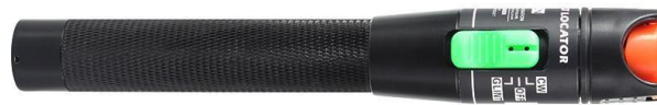
Figure 4.8: Fibre laser pen, or visual fault locator. Injects visible laser beam into fibre, which allows basic alignment and mode matching.
